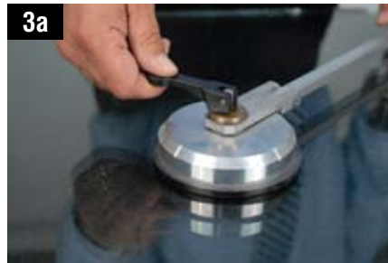
This \frac{3}{4} -inch-thick circular glass lite is ready for further processing on a grinding machine.
