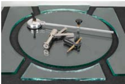
This \frac{3}{4} -inch-thick circular glass lite is ready for further processing on a grinding machine.
