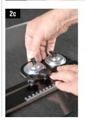
Adjust the glass cutter's transverse handle and simulate the cut. Press slightly against the spring to ensure the cutting head rotates freely and the cutting fluid is applied.
