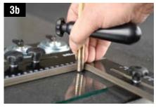
Make the cut, guiding the glass cutter along the simulated cut and applying pressure. Note, the glass cutter must be held in an absolutely vertical position during the entire cutting process.
