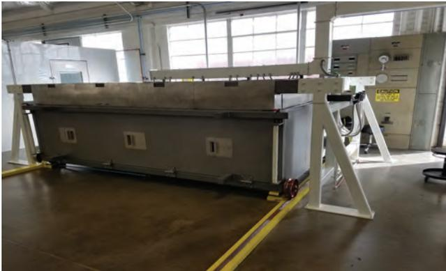
Bending Furnace for Ballistic Aircraft Glass
