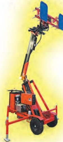
The GM800 & The GM1200 Both have the functions of the GM2000-12. They lift 800 or 1200 pounds respectively to a height of 10 feet. They have a small turning radius and are relatively light weight. Perfect for the **shop, factory & job site**.
