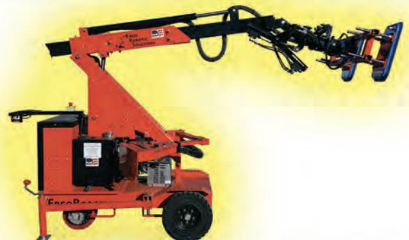
**The GL1200** This model is capable of working with a payload 1200 pounds at a height of 13 feet. It falls between the GM800 and the GM2000-12 in capacity, and is very heavy duty.
