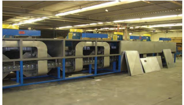
Infrared & Convection Laminating Line
