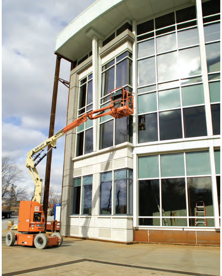
AAMA 501.5, Test Method for Thermal Cycling of Exterior Walls, on a two-story mock-up. Photo courtesy of Architectural Testing.
