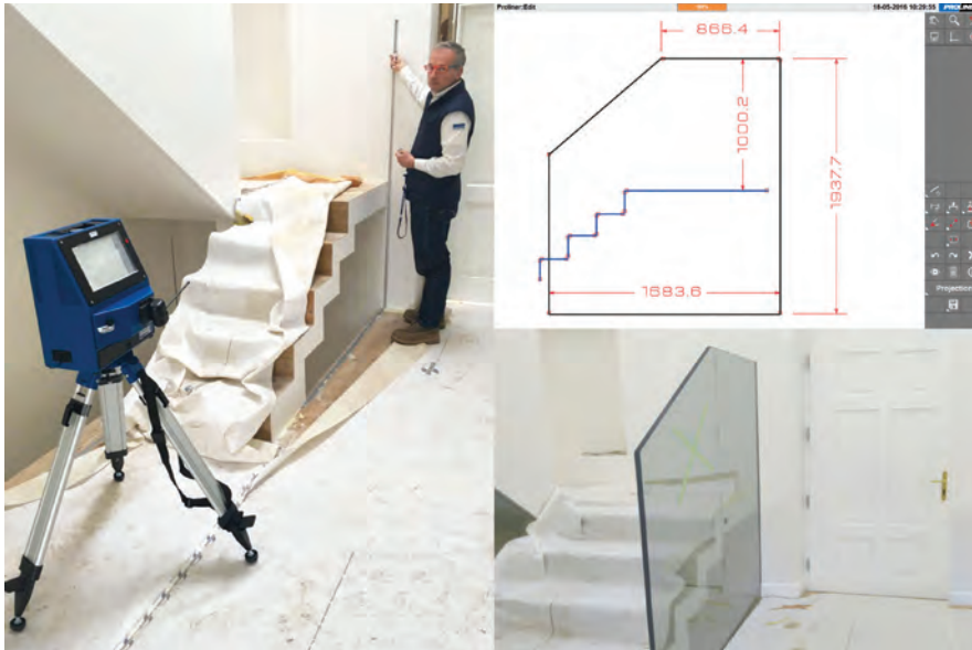
Top: The Proliner digital templating device from Prodim International.
