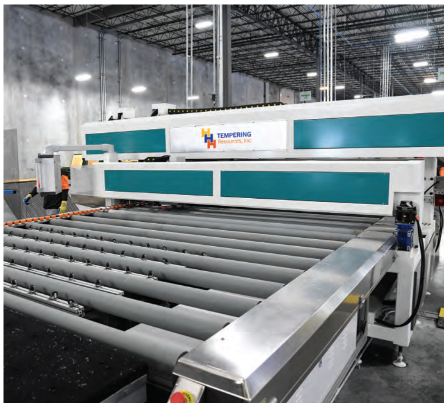
HHH Tempering Resources's 4-Edge Horizontal Glass Grinder. The equipment removes edges and coatings using the four-edge horizontal glass grinding machine, and features a servo motor control system.
