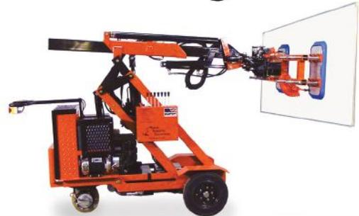
**GM800** The functions of the GM2000-12, it lifts 800 pounds to a height of 10 feet. It has a small turning radius and is relatively light weight.
