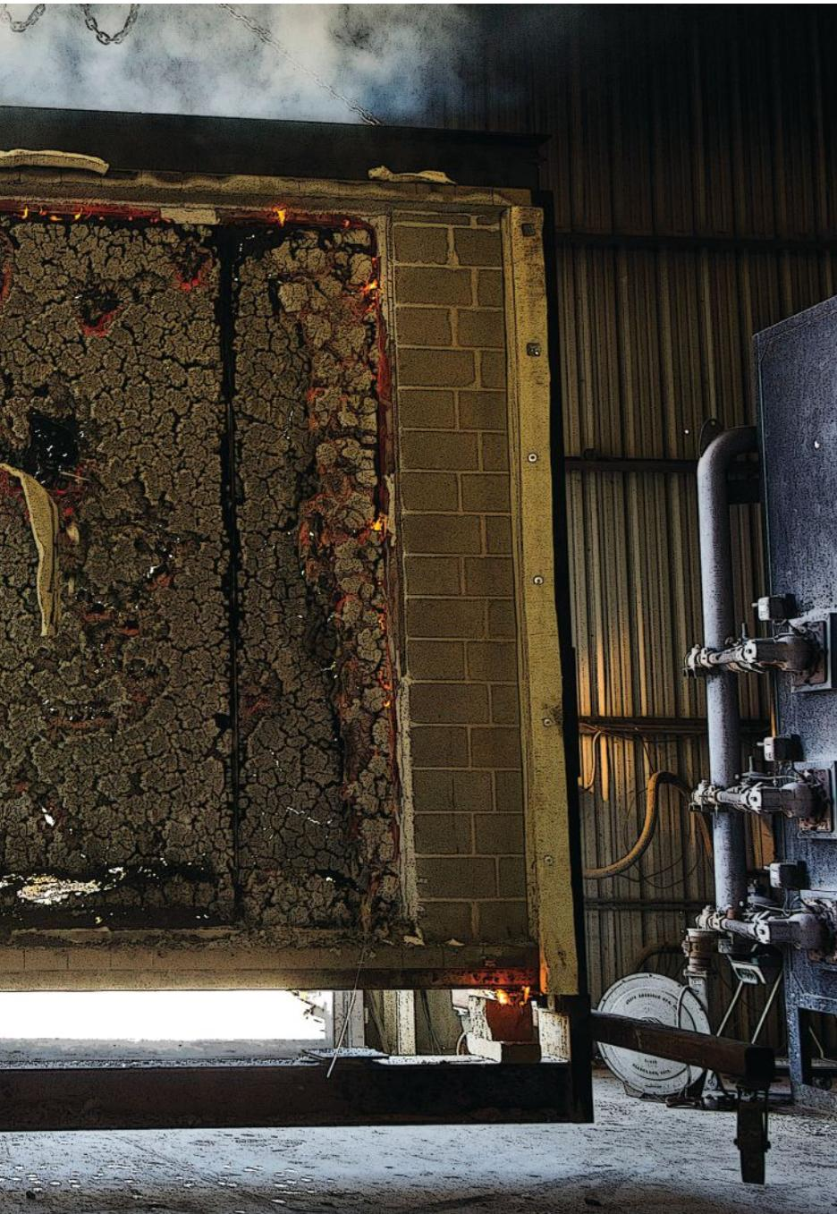
This photo was taken during the two-hour fire-resistive test of SuperLite II-XLB Glazing with GPX Architectural Series Framing from SaftiFirst, safti.com. The test was performed in February 2016 on a 10-foot, 4-inch by 11-foot, 7-inch butt glazed test assembly at the Intertek Testing Services San Antonio Test Facility.
