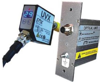
parameters and threshold adjustment. The output of the control unit is a discrete, NPN/PNP that indicates when the signal level exceeds the threshold setting which occurs when viewing the tin-side.
